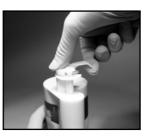
8. Lock the mixing tip in position by slipping the yellow locking cap over the mixing tip and turning clockwise.
